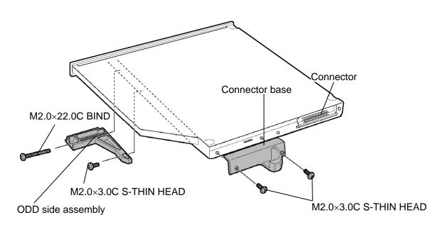
Figure 4-10 Detaching the optical drive assembly
